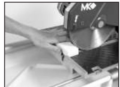
(C) Position the Dressing Stick. Cut 2 or 3 strips from the dressing stick to dress the Blade.
