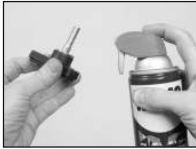
(J) Lubricate the Cutting Head Adjustment Knob.
