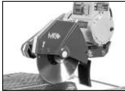
(B) Inspect Diamond Blade for damage.
