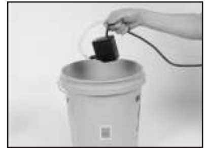
(C) Place Pump into a bucket of water and check flow. If flow exists, go to Step D.
