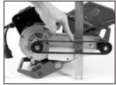
(O) Check Micro-V Belt tension (proper tension 1/8-inch) Repeat steps N and O until proper Micro-V Belt tension is achieved
