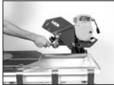
(D) Depress and hold the Shaft Lock pushbutton and remove Retaining Nut and Outer Flange using the Blade Wrench.
