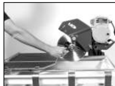
(G) Install Retaining Nut and Outer Flange, depress and hold the Shaft Lock pushbutton and tighten Retaining Nut.
