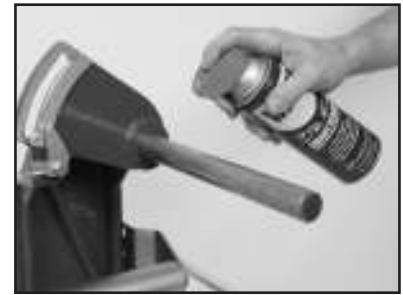
(L) Lubricate the Cutting Head Pivot Shaft.
