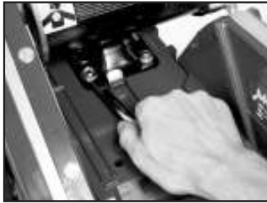
(P) Tighten the four motor mounting bolts
