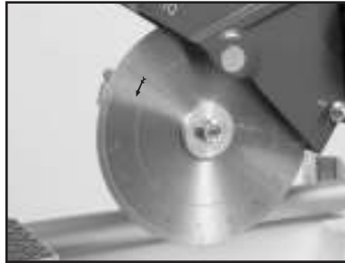
(B) Check for proper blade rotation.
