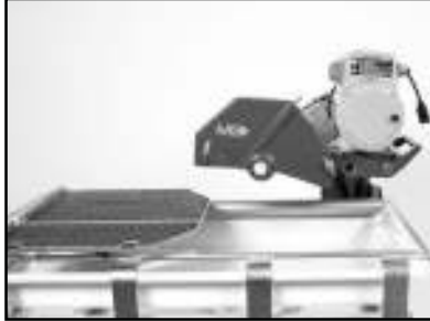
(A) Position Movable Cutting Table to the front of the saw.
