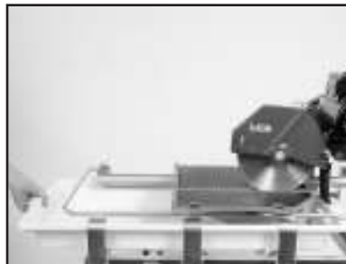
(B) Remove Water Basin, place saw on stand
