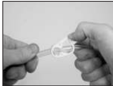
(B) Reduce cooling flow by Pressing down on the Flow Adjusting Clamp.
