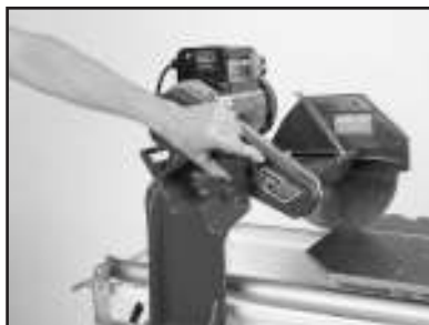
(A) Loosen Cutting Head Adjusting Knob.
