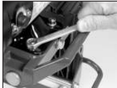
(E) Verify all motor mounting Bolts are tight.
