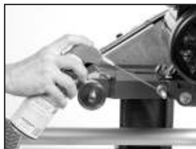
(H) Lubricate the Blade Guard Pivot Shaft.
