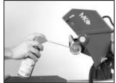
(C) Lubricate the Arbor Shaft.
