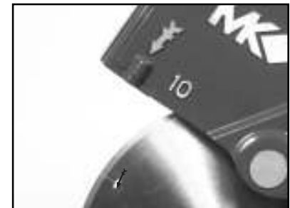
(F) Verify the Blade is seated on the Blade Shaft and direction of rotation is correct.
